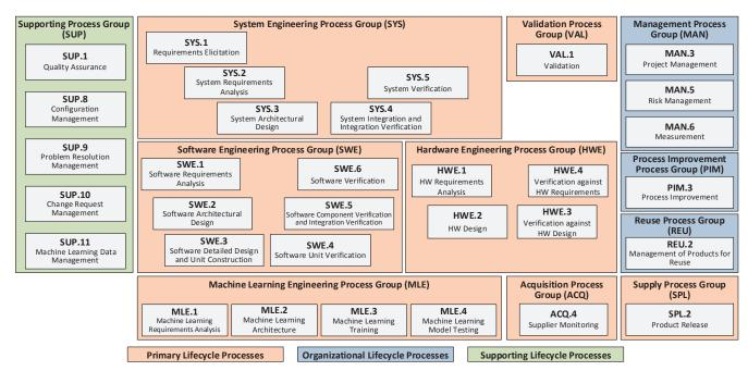
ASPICE defines in this criteria and 2 dimensions the overview of SW Project, to determinate the capability of SW developing process & process improvement.
